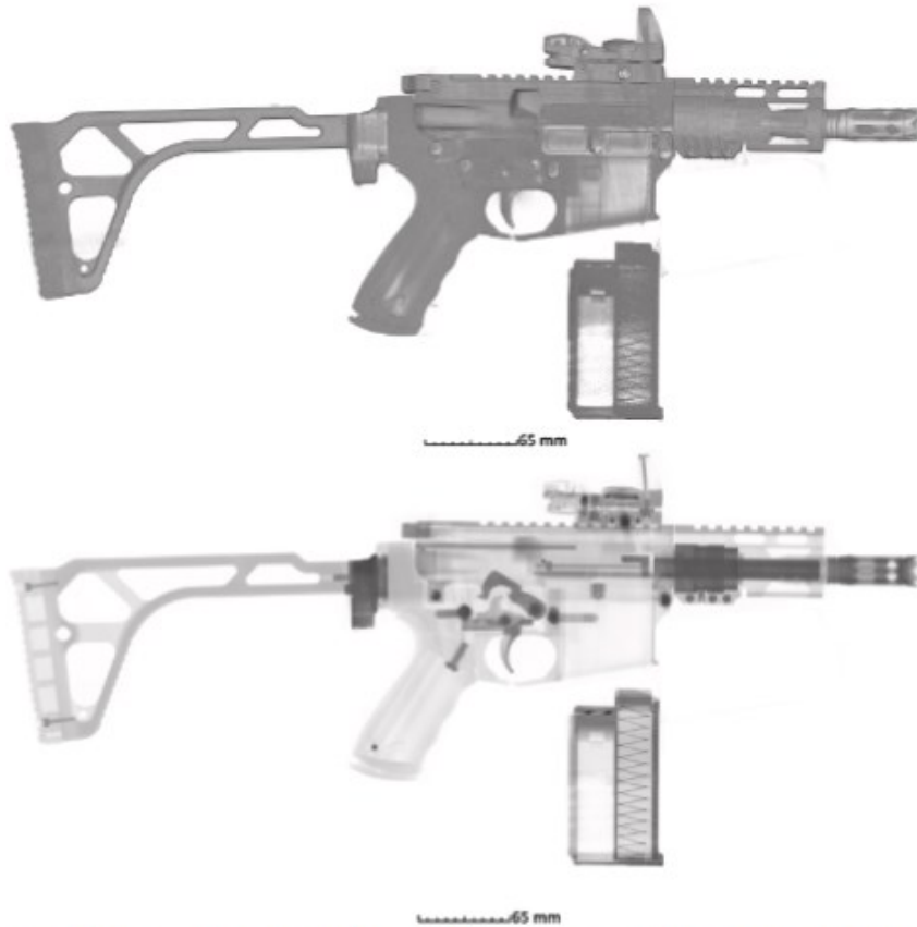
Fig. 4. Right lateral views of the 3D volume-rendered micro-CT scan (top) and X-ray (bottom) of JRM-02.
