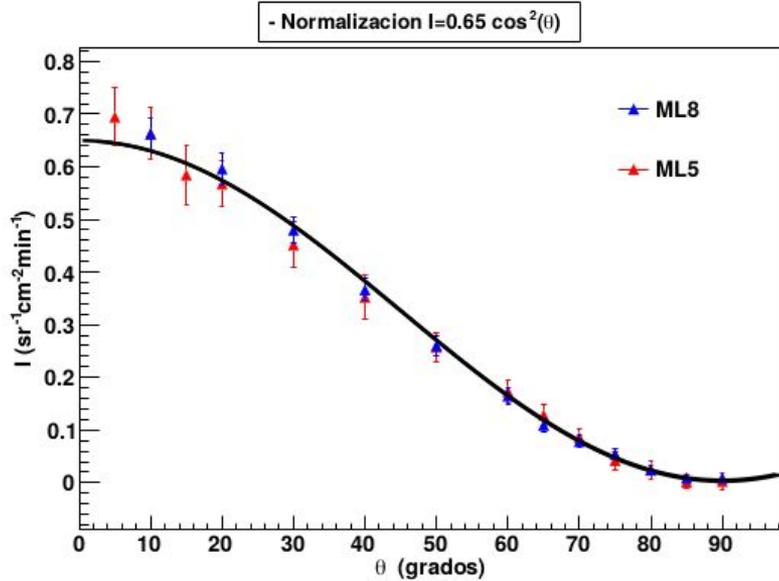
Open sky muon flux measurement
